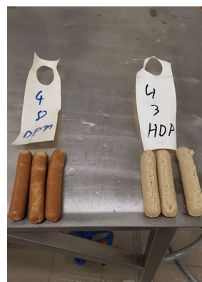
43 HDP. Wheels in the peeler might have damaged the not-firm surface of the sausages.
