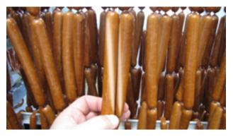
The second limitation of the strand load is the weight of the filled strand. It's not just bodybuilders beside the stuffing machine who need to carry the filled strands from the conveyor chain to the trolley or to the automatic processing lines. The final weight of the strand can limit its load.
