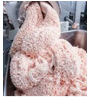
Picture 2: Pre-grinding at low temperature does not show an indication of fat quality.
