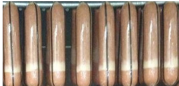
Picture 3: Melted fat on top on the gel separation is hardened after cooling down.
